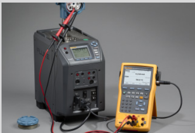
Testing a temperature transmitter using a dry well calibrator
