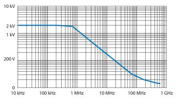
Voltage vs. Frequency Derating Curve TT-HV 400
